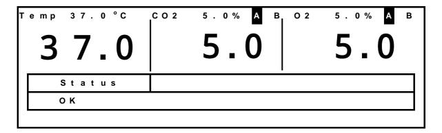
(When the line needs to be switched from  $N_2$  (or  $O_2$ ) gas cylinder A to B, press the Down Cursor Key for 3 seconds.)
